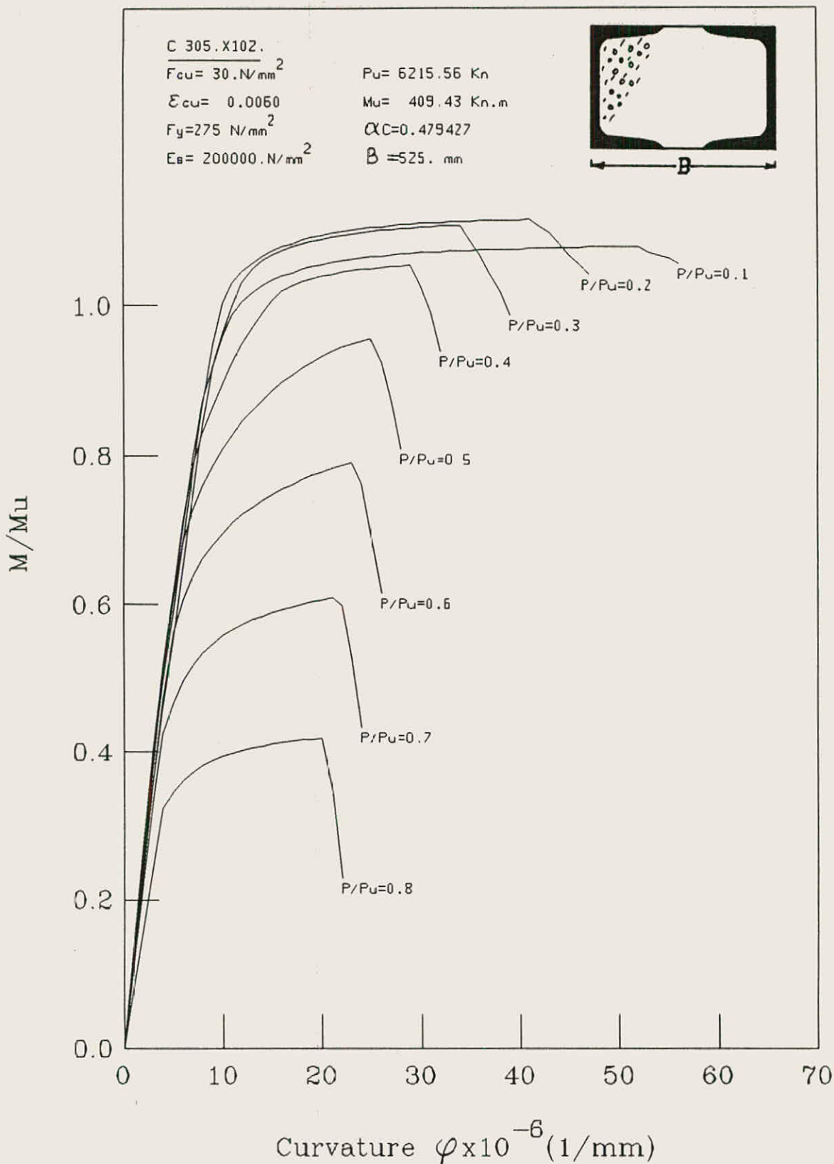
FIG. (C-11): MOMENT-CURVATURE-THRUST CURVES FOR BATTENED COMPOSITE COLUMN UNDER UNIAXIAL BENDING MOMENT ABOUT MINOR AXIS .
